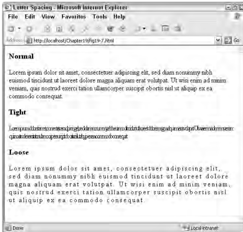
Figure 19-7: The letter-spacing property does exactly as its name indicates, adjusts the spacing between letters.
