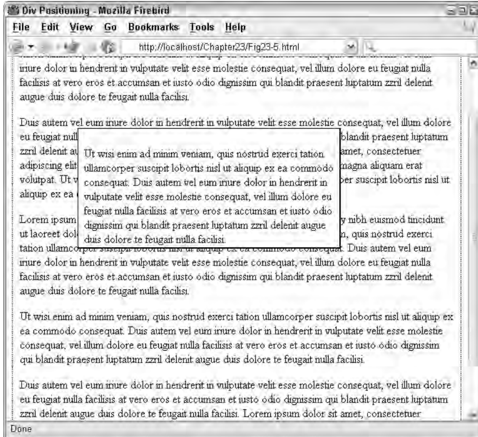
Figure 23-5: Elements using the fixed positioning model do not scroll in the view port, as shown when this document scrolls.
