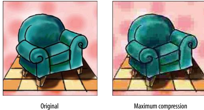
Figure 21-9. JPEG compression discards image detail to achieve smaller file sizes. At high compression rates, image quality suffers, as shown in the image on the right.
