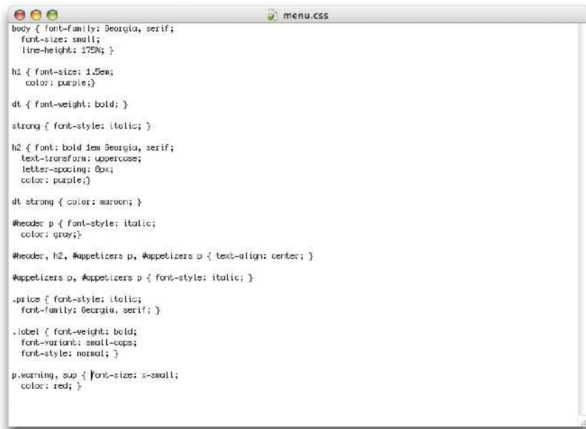
Figure 13-28. External style sheets contain only CSS rules and comments in a plain text document.
