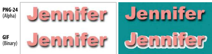
Figure 21-27. The difference between binary and alpha transparency becomes very clear when the background color of the page changes.
