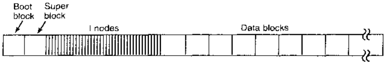
Figure 10-31. Disk layout in classical UNIX systems.
