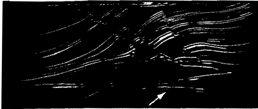
FIGURE 1.19 Cross-sectional image of a seismic model. The arrow points to a hydrocarbon (oil and/or gas) trap. (Courtesy of Dr. Curtis Ober, Sandia National Laboratories.)
