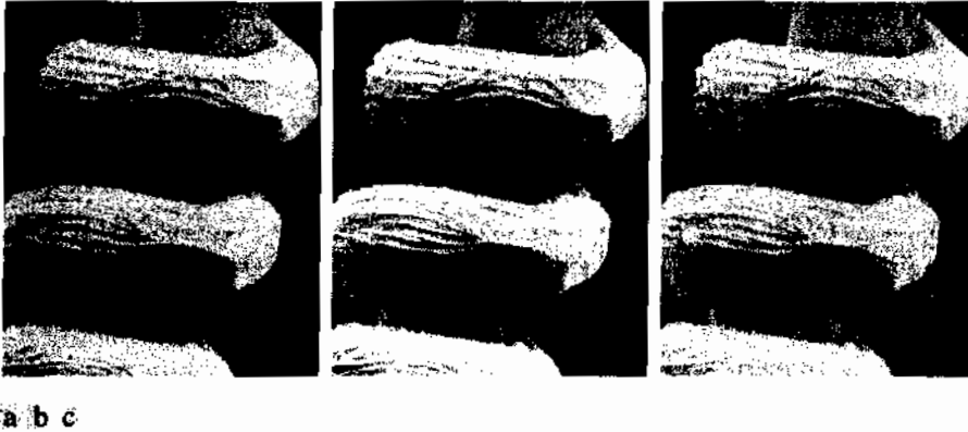
FIGURE 3.27 (a) SEM image of a tungsten filament magnified approximately 130 \times . (b) Result of global histogram equalization. (c) Image enhanced using local histogram statistics. (Original image courtesy of Mr. Michael Shaffer, Department of Geological Sciences, University of Oregon, Eugene.)
