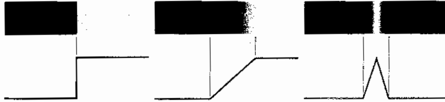
FIGURE 10.8 From left to right, models (ideal representations) of a step, a ramp, and a roof edge, and their corresponding intensity profiles.
