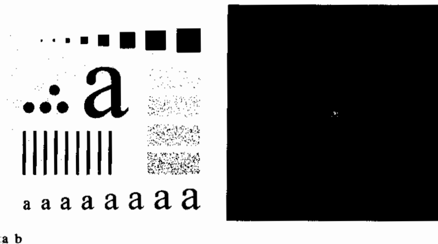
FIGURE 4.41 (a) Test pattern of size 688 \times 688 pixels, and (b) its Fourier spectrum. The spectrum is double the image size due to padding but is shown in half size so that it fits in the page. The superimposed circles have radii equal to 10, 30, 60, 160, and 460 with respect to the full-size spectrum image. These radii enclose 87.0, 93.1, 95.7, 97.8, and 99.2% of the padded image power, respectively.
