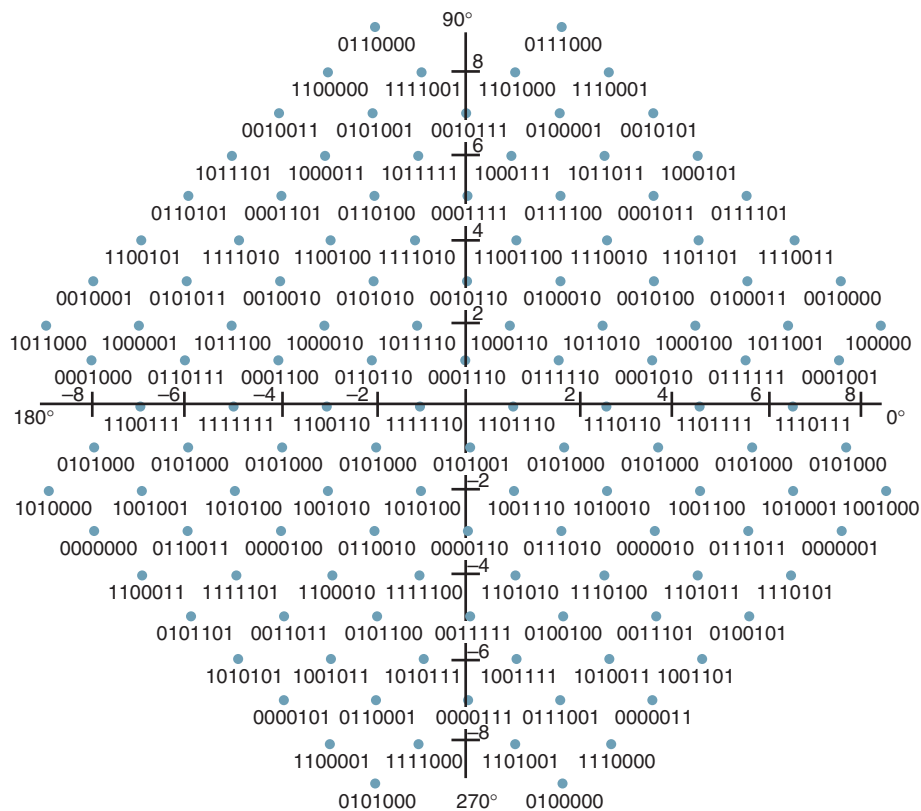
FIGURE 45 128-Point QAM TCM constellation
