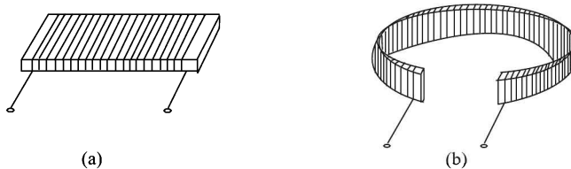
Fig. 6.5 Wire-wound resistance elements on: (a) straight insulating card and (b) circular insulating card.
