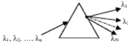
FIGURE 9 A dispersive prism spatially separates different wavelengths. This represents demultiplexing. Reversing the directions of the arrows illustrates combining of different wavelengths. This is multiplexing.
