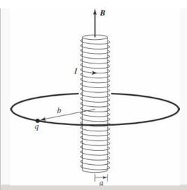
Figure 4.16: Charged bead on a circular ring through which a long solenoid passes.
