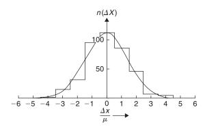
**FIGURE 15.1** The statistical distribution of the successive displacements,  $\Delta x$ , of a Brownian particle immersed in water:  $(\Delta x)_{\text{r.m.s.}} \simeq 1.45 \,\mu$ .
