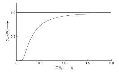
**FIGURE 6.4** The vibrational specific heat of a gas of diatomic molecules. At  $T = \Theta_{\nu}$ , the specific heat is already about 93 percent of the equipartition value.
