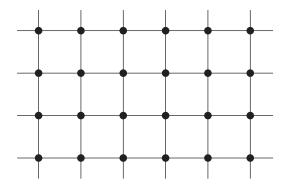
**FIGURE 13.16** A finite square lattice with n = 4 rows and m = 6 columns. In view of the periodic boundary conditions, sites on the leftmost column interact with sites on the rightmost column and the bottom row interacts with the top row.
