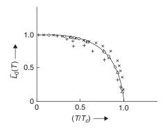
**FIGURE 12.7** The spontaneous magnetization of a Weiss ferromagnet as a function of temperature. The experimental points (after Becker) are for iron  $(\times)$ , nickel (o), cobalt  $(\Delta)$ , and magnetite (+).
