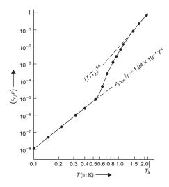
**FIGURE 7.17** The normal fraction  $(\rho_n/\rho)$ , as obtained from experimental data on (i) the velocity of second sound and (ii) the entropy of liquid He II (after de Klerk, Hudson, and Pellam, 1953).
