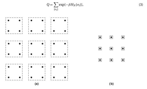
**FIGURE 14.1** A block–spin transformation, with l=2 and d=2. The original lattice (a) has N = 36 spins, the transformed one (b) has N' (= 9); after rescaling, the latter looks very much the same as the former, especially in the limit  $N, N' \to \infty$ .
