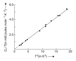
**FIGURE 7.16** A plot of  $(C_V/T)$  versus  $T^2$  for KCl, showing the validity of the Debye  $T^3$ -law. The experimental points are from Keesom and Pearlman (1953).
