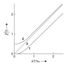
**FIGURE 3.4** The mean energy  $\langle \varepsilon \rangle$  of a simple harmonic oscillator as a function of temperature. 1, the Planck oscillator; 2, the Schrödinger oscillator; and 3, the classical oscillator.
