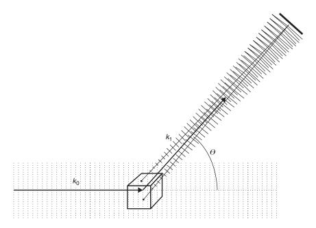
**FIGURE 10.7** Scattering from two particles. The incident wavevector is  $k_0$ , the scattered wavevector toward the detector is  $k_1$ , and the wavevector transfer is  $k = k_1 - k_0$ . Since  $|k_1| = |k_0|$  for quasielastic scattering, the magnitude of the wavevector transfer is  $k = 2k_0 \sin(\theta/2)$ , where  $\theta$  is the angle between  $k_0$  and  $k_1$ .
