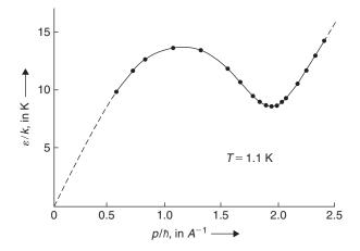
FIGURE 7.18 The energy spectrum of the elementary excitations in liquid He II at 1.1K [after Yarnell et al. (1959)]; the dashed line emanating from the origin has a slope corresponding to the velocity of sound in the liquid, namely (239  $\pm$  5) m/s.
