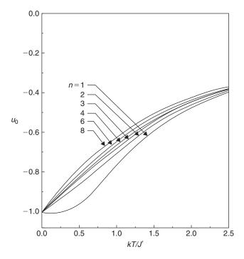
**FIGURE 13.6** The normalized energy  $u_0 = U_0/NnJ'$  of a one-dimensional chain as a function of the temperature parameter kT/J' for several values of n (after Stanley, 1969a,b). Note that for this classical model, the slopes as  $T \to 0$  are given by the equipartition theorem for n-1 degrees of freedom per spin.
