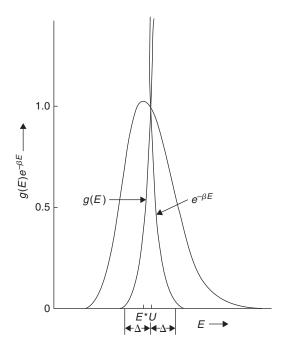
**FIGURE 3.3** The actual behavior of the functions g(E),  $e^{-\beta E}$ , and  $g(E)e^{-\beta E}$  for an ideal gas, with N=10. The numerical values of the functions have been expressed as fractions of their respective values at E=U.
