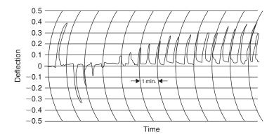
**FIGURE 3.16** A typical record of the reversed nuclear magnetization (after Purcell and Pound, 1951). On the left we have a deflection corresponding to normal, equilibrium magnetization  $(T \sim 300\,\mathrm{K})$ ; it is followed by the reversed deflection (corresponding to  $T \sim -350\,\mathrm{K}$ ), which decays through zero deflection (corresponding to a passage from  $T = -\infty$  to  $T = +\infty$ ) toward the new equilibrium state that again has a positive T.
