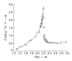
FIGURE 7.5 The specific heat of liquid He<sup>4</sup> under its own vapor pressure (after Keesom and coworkers).
