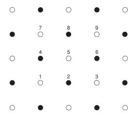
FIGURE 14.4 A section of the two-dimensional Ising lattice. The summed-over spins are denoted by open circles, the remaining ones by solid dots. To begin with, we concentrate on the summation over  $\sigma_5$ .
