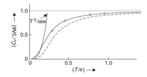
**FIGURE 7.14** The specific heat of a solid, according to the Einstein model: — — , and according to the Debye model: —. The circles denote the experimental results for copper.
