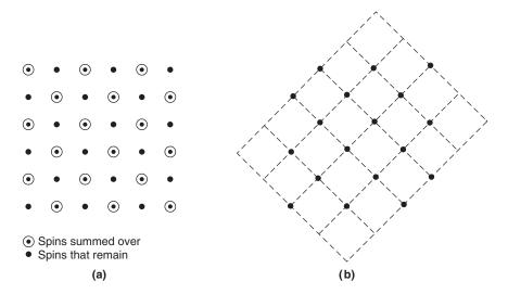
**FIGURE 14.2** A scale transformation by "decimation," with  $l = \sqrt{2}$  and d = 2. The original lattice (a) has N (= 36)spins, the transformed one (b) has N' (= 18); the latter is yet to be rescaled (and rotated through an angle  $\pi/4$ ) so that it looks very much the same as the former, especially in the limit  $N, N' \to \infty$ .
