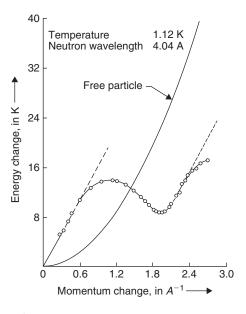
**FIGURE 7.19** The energy spectrum of the elementary excitations in liquid He II at 1.12K (after Henshaw and Woods, 1961); the dashed straight lines have a common slope corresponding to the velocity of sound in the liquid, namely  $237\,\mathrm{m/s}$ . The parabolic curve rising from the origin represents the energy spectrum,  $\varepsilon(p)=p^2/2m$ , of free helium atoms.
