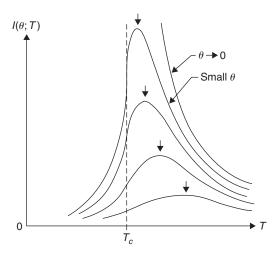
**FIGURE 12.13** Schematic plot of the elastic scattering intensity of neutrons scattered at an angle  $\theta$  from a magnetic system, such as iron, in the vicinity of the critical point  $T_c$ . The small arrows mark the smoothly rounded maxima (at fixed  $\theta$ ) which occur at a temperature  $T_{\sf max}(\theta)$  that approaches  $T_c$  as  $\theta \to 0$ .
