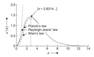
**FIGURE 7.13** The spectral distribution of energy in the blackbody radiation. The solid curve represents the quantum-theoretical formula of Planck. The long-wavelength approximation of Rayleigh–Jeans and the short-wavelength approximation of Wien are also shown.
