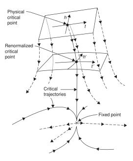
**FIGURE 14.5** The parameter space of a physical system, showing critical trajectories (solid lines) flowing into the fixed point. The subspace of the relevant variables, t and h, is everywhere "orthogonal" to these trajectories (on all of which t=h=0); the critical trajectories differ from one another only in respect of irrelevant variables that vanish as the fixed point is approached. The dashed lines depict that part of the flow in which the relevant variables play a decisive role.
