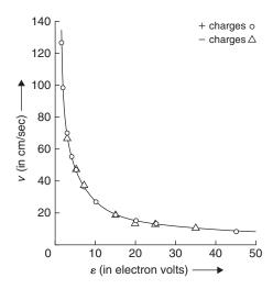
**FIGURE 11.6** The velocity–energy relationship of the vortex rings formed in liquid helium II (after Rayfield and Reif, 1964). The points indicate the experimental data, while the curve represents the theoretical relationship based on the "quantum of circulation" h/m.
