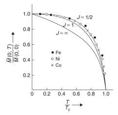
**FIGURE 12.4** Spontaneous magnetization of iron, nickel, and cobalt as a function of temperature. Theoretical curves are based on the Weiss theory of ferromagnetism.
