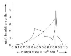
**FIGURE 7.15** The normal-mode frequency distribution  $g(\omega)$  for aluminum. The solid curve is derived from x-ray scattering measurements [Walker (1956)] while the dashed curve represents the corresponding Debye approximation.
