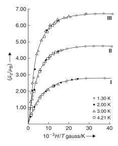
**FIGURE 3.9** Plots of  $\overline{\mu}_z/\mu_B$  as a function of H/T. The solid curves represent the theoretical results, while the points mark the experimental findings of Henry (1952). Curve I is for potassium chromium alum  $(J=\frac{3}{2},g=2)$ , curve II for iron ammonia alum  $(J=\frac{5}{2},g=2)$ , and curve III for gadolinium sulphate octahydrate  $(J=\frac{7}{2},g=2)$ .
