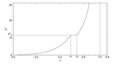
FIGURE 16.3 Sketch of the equilibrium phase diagram for hard spheres in three dimensions. The horizontal axis is the volume fraction  $\eta = \pi nD^3/6$  and the vertical axis is the scaled pressure  $P^* = PD^3/kT$ . There are two equilibrium phases: a low-density fluid phase for  $0 < \eta < \eta_I$  and a high-density solid phase for  $\eta_S < \eta < \eta_{CD}$ .
