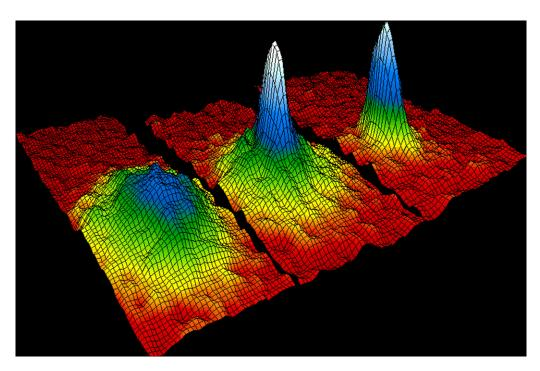
FIGURE 7.9 Time-of-flight images from the first observation of Bose-Einstein condensation in a dilute vapor of <sup>87</sup>Rb by Anderson et al. (1995) at temperatures just above and below the phase transition temperature. The anisotropic pattern of the Bose-condensed fraction is evident; compare to Figure 7.8. Courtesy of NIST/JILA/University of Colorado.
