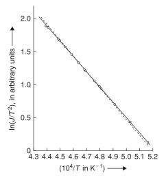
FIGURE 8.6 Thermionic current from tungsten as a function of the temperature of the metal. The continuous line corresponds to  $r = \frac{1}{2}$  while the broken line corresponds to r = 0, r being the reflection coefficient of the surface.
